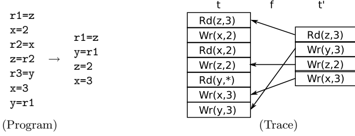
Fig. 4. Transformation of a program as a transformation on traces
